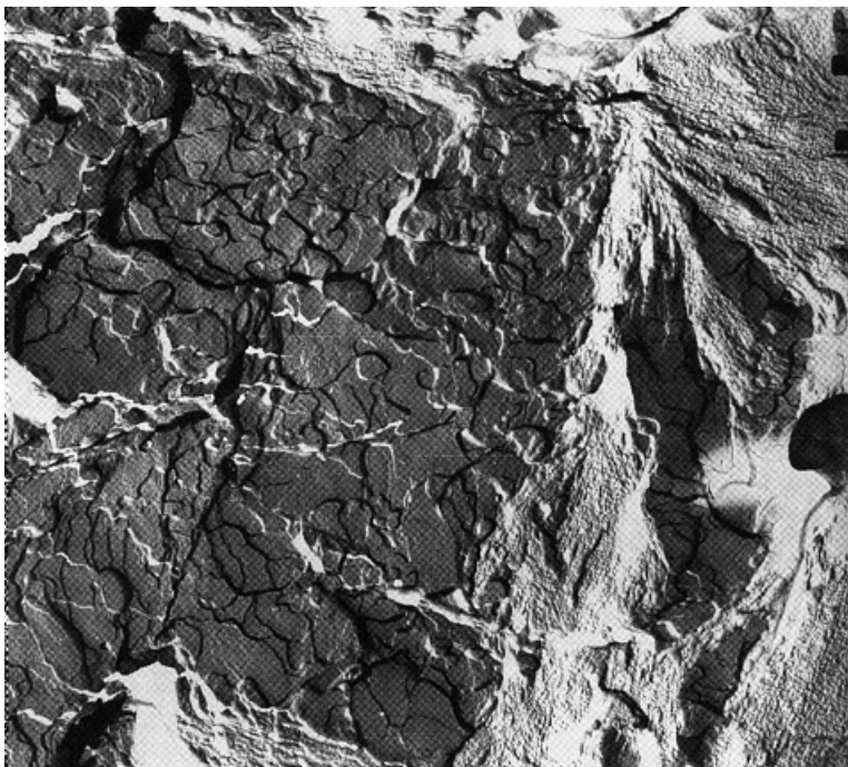
Figure 6.14 Surface replica of polyoxymethylene fractured at liquid nitrogen temperatures. Lamellae at lower left are oriented at an angle to the fracture surface. Lamellae elsewhere are nearly parallel to the fracture surface, being stacked up like cards or dishes in the bulk state. These structures closely resemble stacks of single crystals, and they have led to ideas about chain folding in bulk materials (34).
